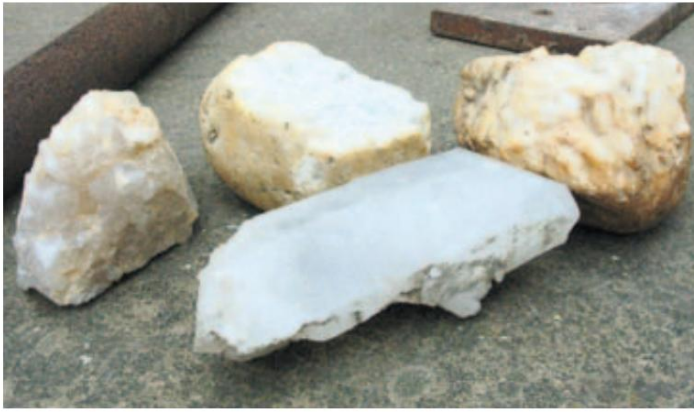
Fig. 5: The crystal structure of pebbles (quartz or rock crystal, left) and orthoclase (right) differs
