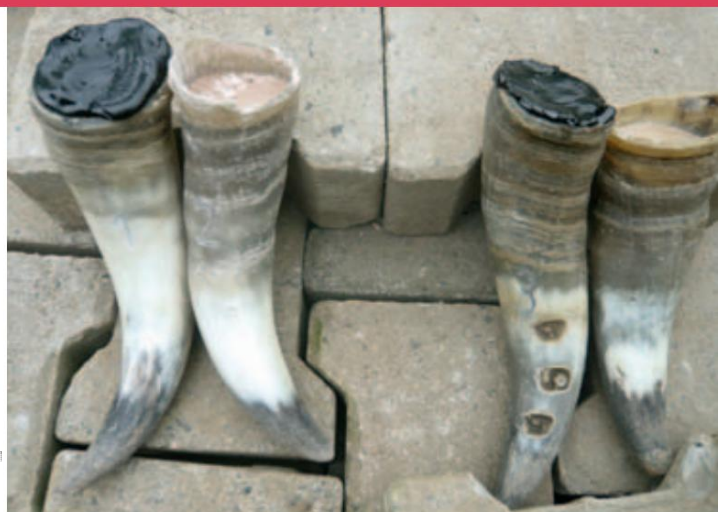
Figure 2: Preparation with orthoclase + soil or only Orthoclase (left) and pebble + earth or only pebbles (right)
