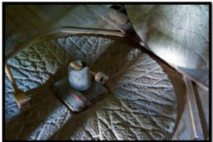
Figure 35 The inner faces of the French Burr mill stones. Image courtesy of Andrew Turner.
