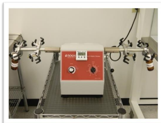
Figure 7. The Wrist O Matic Shaker Agitation Machine. It creates a vortex and shakes the dilution vertically at the same time at approx. 200 times per minute depending on the setting chosen.
