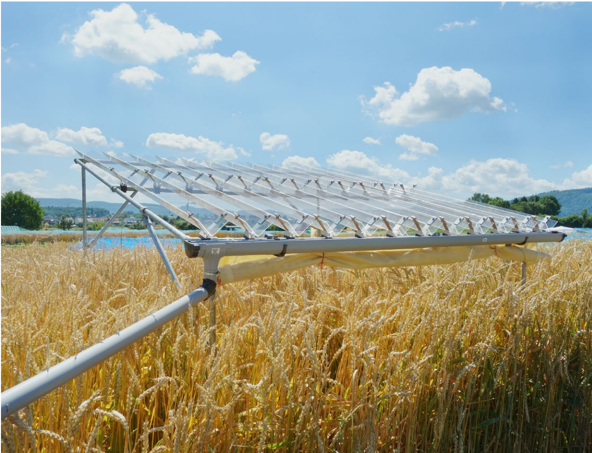
DOK trial plots with wheat and rainout shelters to investigate drought effects on soil biodiversity.
